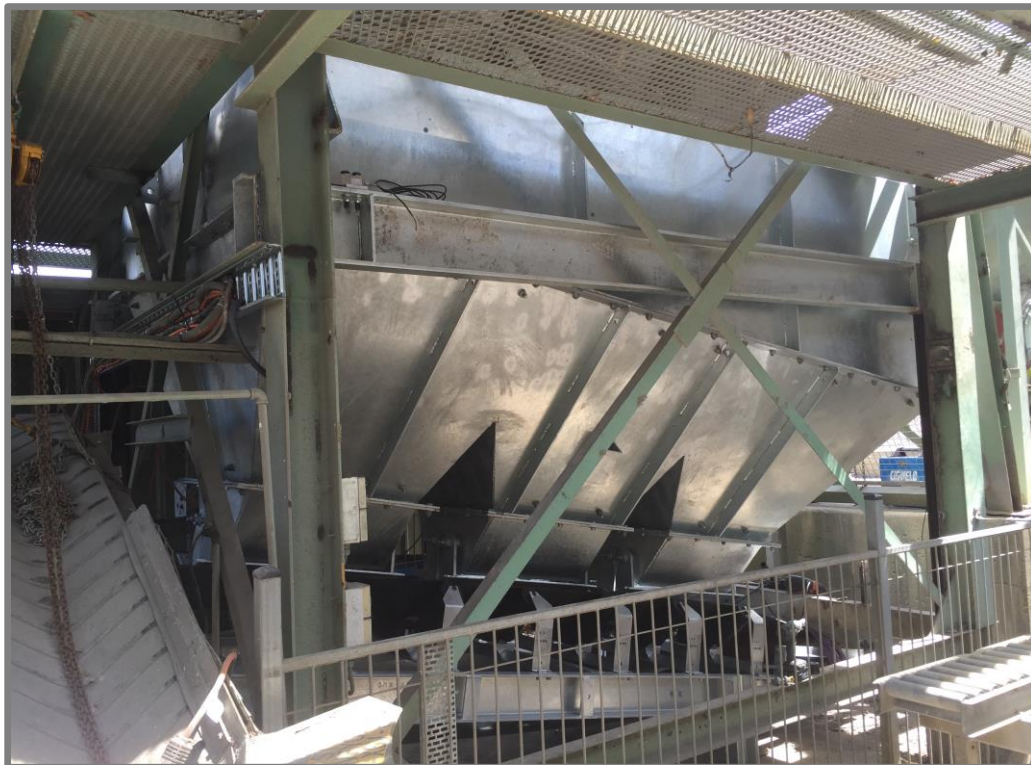
Fully galvanized aggregate weigh bins and conveyor systems
