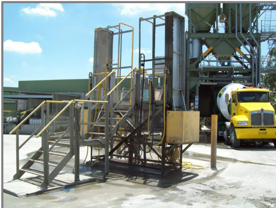
Design and manufacture of fully galvanized fixed or air operated slump stands (single or double)
